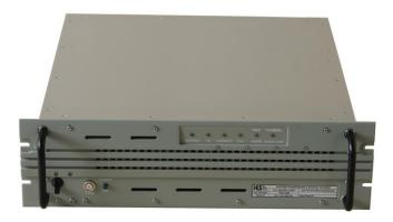
The ASV2000 is an "UHF Integrated Cositing Unit" designed with the aim to improve the technical characteristics of UHF systems. It is used to improve the filtering capabilities of such systems, both in transmission and in reception, and to increase the transmitted RF power. A high selectivity, agile filter is designed to allow simultaneous operation of a large number of transceivers operating in a co-located environment. Its main features are listed below:
